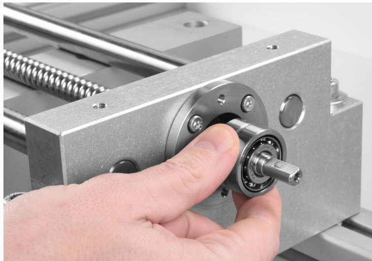
Figure 35: Removing the two angular contact bearings.
