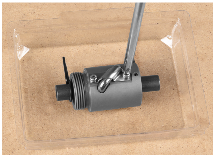
Figure 27: Unscrewing the screws of the return pipe holder on the ball nut.
