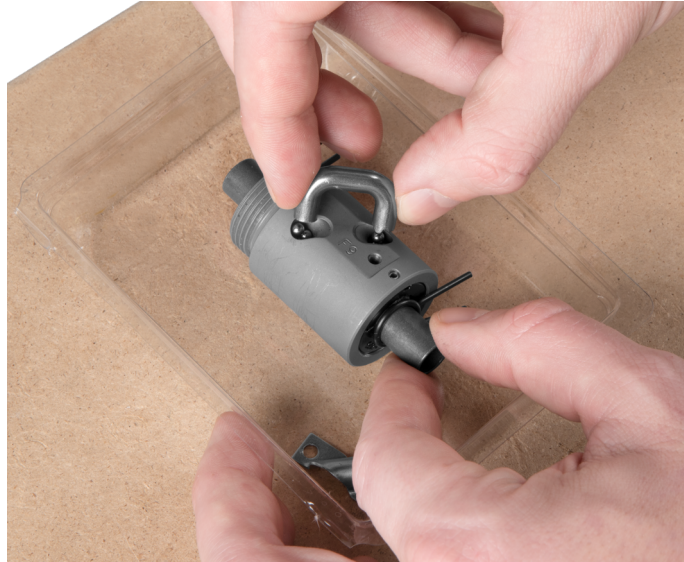
Figure 28: Removing the return pipe.
