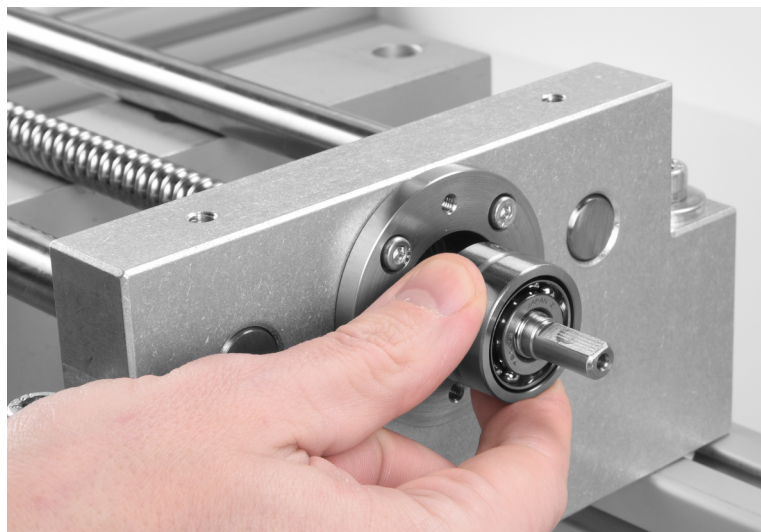
Figure 37: Inserting the angular contact ball bearings in the flange base.
