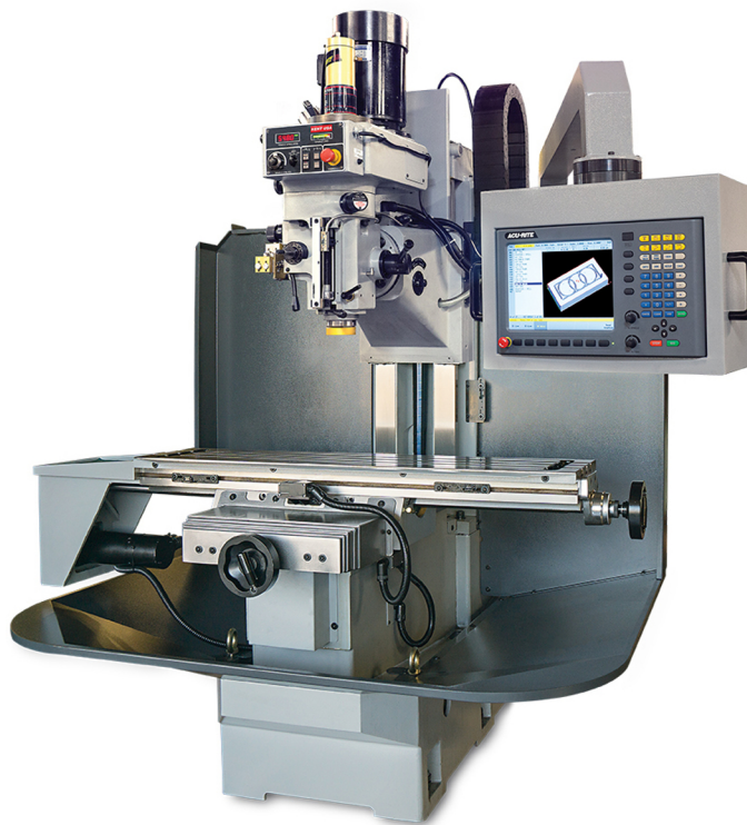
Figure 21: Linear bearings and ball screws are commonly used for horizontal and vertical movement in CNC mills.
