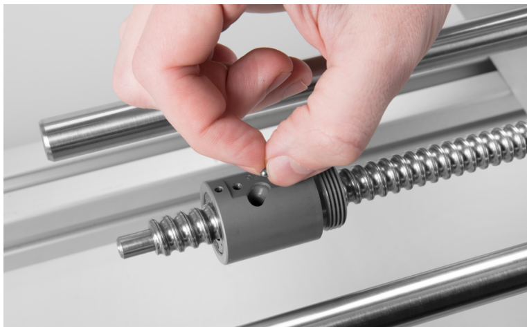
Figure 31: Inserting the balls in the ball nut.
