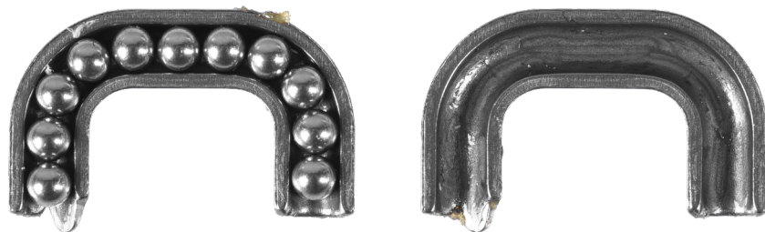
Figure 30: Filling one half of the return pipe with balls.
